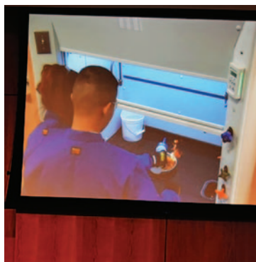
View from above: what is going on in the hood is shown on a large screen above it thanks to cameras pointing into the hood.
