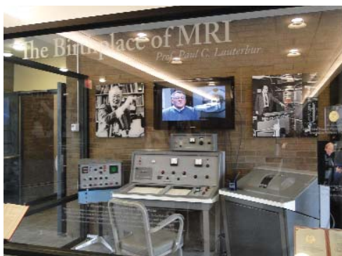
Dr. Paul Lauterbur used the Varian A-60 exhibited here to demonstrate the proof-of-principle that NMR could generate multi-dimensional images.
